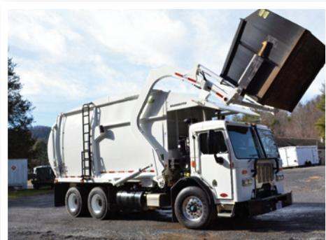
*The biodegradable soy-based hydraulic fluid is used extensively in many of the 200+ pieces of equipment used throughout the park, such as this large refuse compactor truck.*
