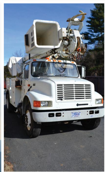
*Another large piece of maintenance equipment utilizing soy-based hydraulic fluid is this bucket lift truck used in reaching high trouble spots such as utility poles or for tree trimming.*
