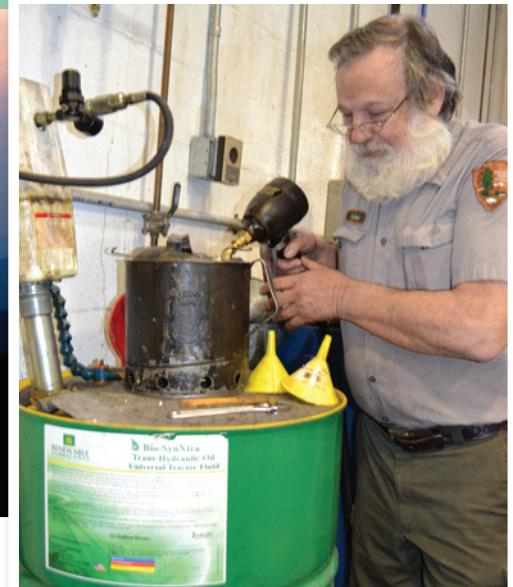
*Kenneth Judd, mobile equipment servicer, is a big proponent of soy-based hydraulic fluid used in SNP hydraulic equipment and as transmission fluid because it is biodegradable and easier to clean up*
